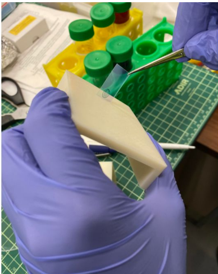
Fig14:Insert the sensor into the cover of the prototype through the hole
